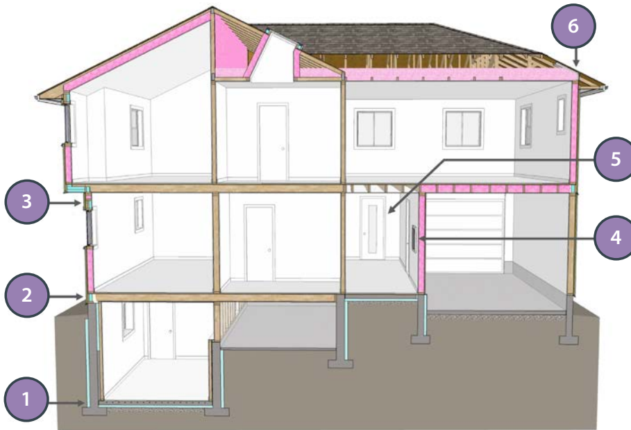
Figure 2: Typical Problem Areas for Insulation Continuity
